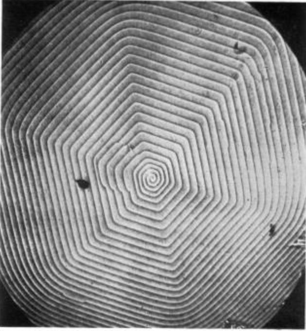
Fig. 3.5 A growth spiral on a crystal of SiC grown from the vapour (Verma 29 ).
