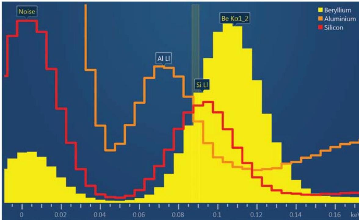
*Spectra from Al, Si and Be showing separation of K and L peaks from baseline noise.*
