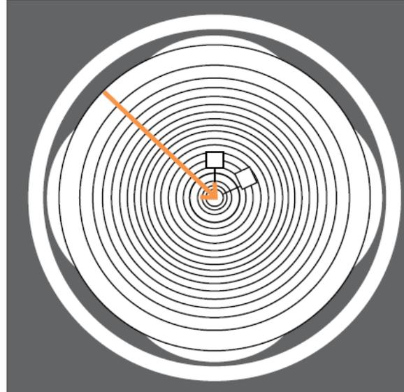
Most common SDD shapes: Tear-drop with integrated FET. The FET is at the periphery of the design meaning greater charge cloud travel distance than required for a radial design B) where an external FET is bonded to a central anode.
