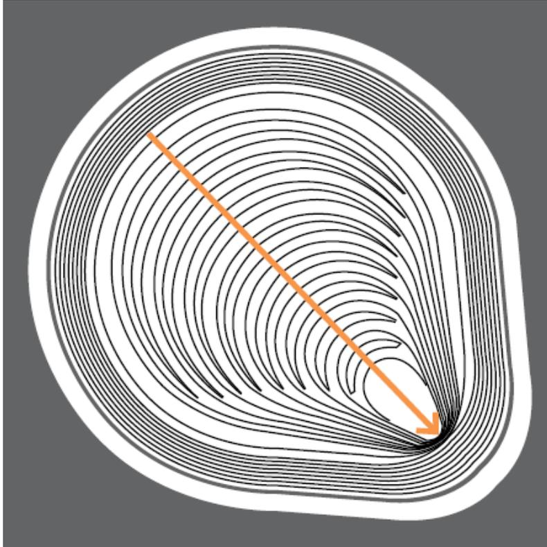
*Tear-drop shape (to protect FET) with integrated FET, is subject to charge collection issues, and electrical characteristics causing **resolution & peak shifts, plus size limitations***
