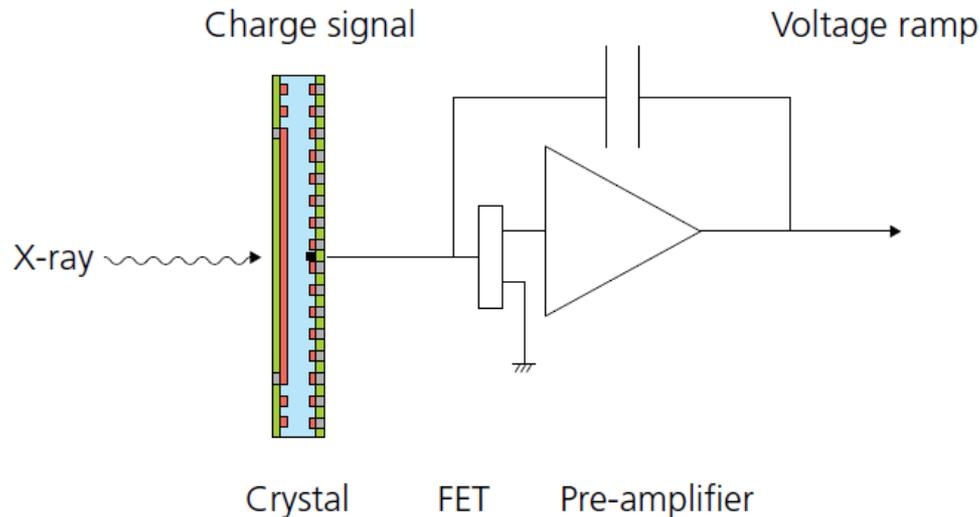
The charge which accumulates at the anode is converted to a voltage by the FET preamplifier. During operation, charge is built up on the feedback capacitor.
