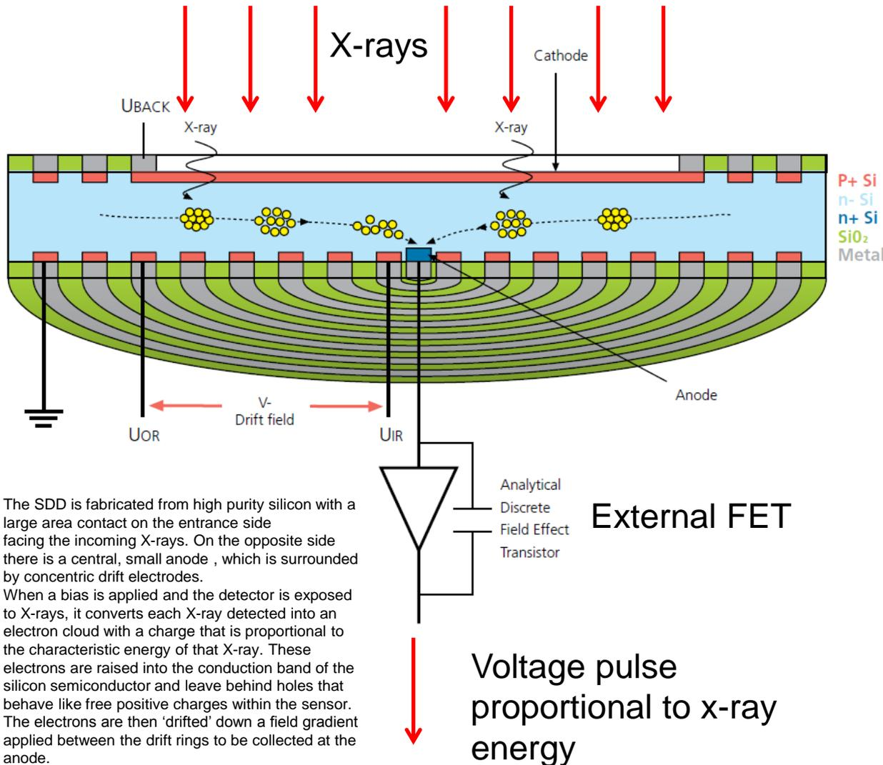
The SDD is fabricated from high purity silicon with a large area contact on the entrance side facing the incoming X-rays. On the opposite side there is a central, small anode, which is surrounded by concentric drift electrodes.
