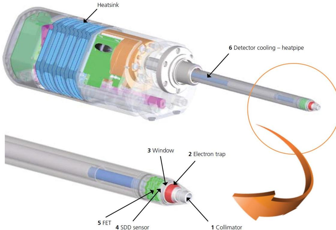
1. **The collimator** prevents stray X-rays entering the detector.
