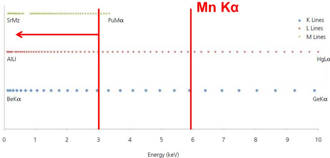
Showing the energy of the major lines for K, L and M series for all elements. Note that the resolution at Mn (5.9KeV), peaks are well separated. However, X-ray lines are closer together at lower energies, notably below 3kV where overlaps become significant. Thus **resolution and deconvolution performance at low kV is critical**
