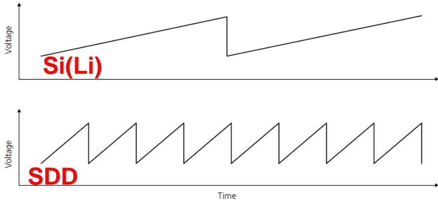
Leakage current (gradient on the voltage ramp) is larger for SDDs but **since process time is shorter, leakage current is of lesser importance** than with Si(Li) detectors
